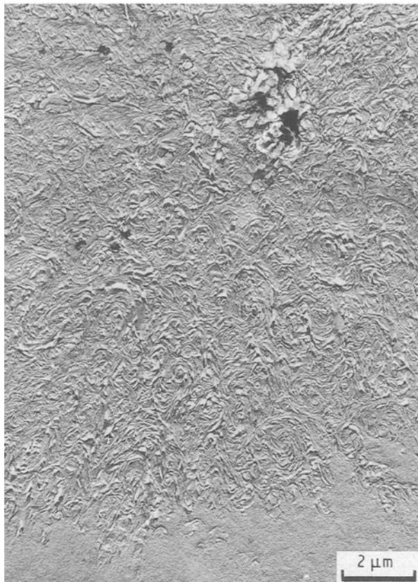
Figure 9 A spherulite of  $\gamma$ -PVF<sub>2</sub> (Solef 1010) grown at 172°C as seen when viewed down the radius. Thick film, two-stage replica.
